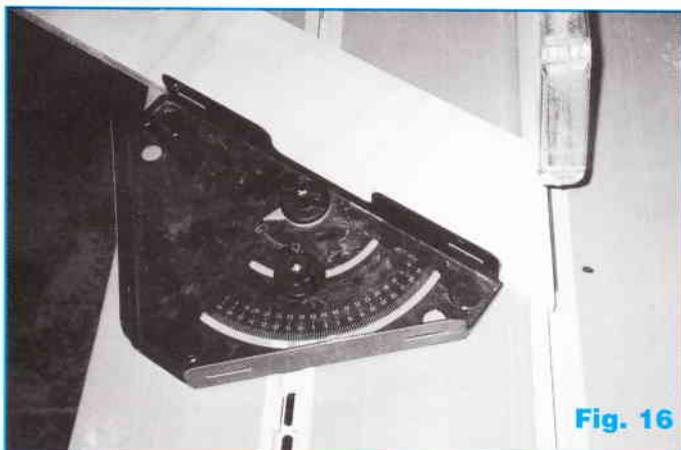
Mitre cut one end of the other two pieces but this time set the protractor to  $12.3^\circ$  using the same scale. This will create two "corners".
