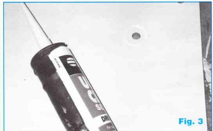
Use a caulk gun if you have one, to squeeze out a bead of silicon around each hole (**Fig. 3**) then lay each mesh square in place on the bead.
