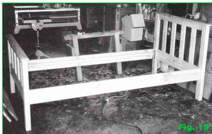
**10** Check that the bed is square and measure the distance between the side rails. It should be about 930 mm. Cut the six slats (E) using the Workcentre in the crosscut mode (Fig. 20).
