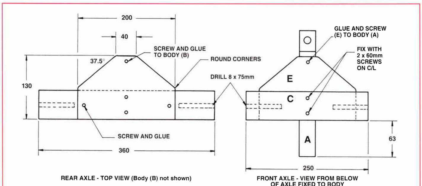
**FIGURE 7: AXLES AND BRACES**
