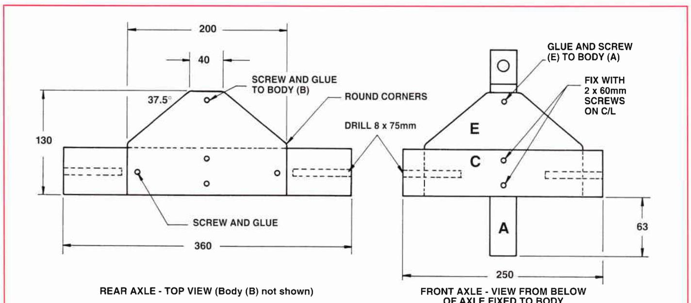
FIGURE 7: AXLES AND BRACES
